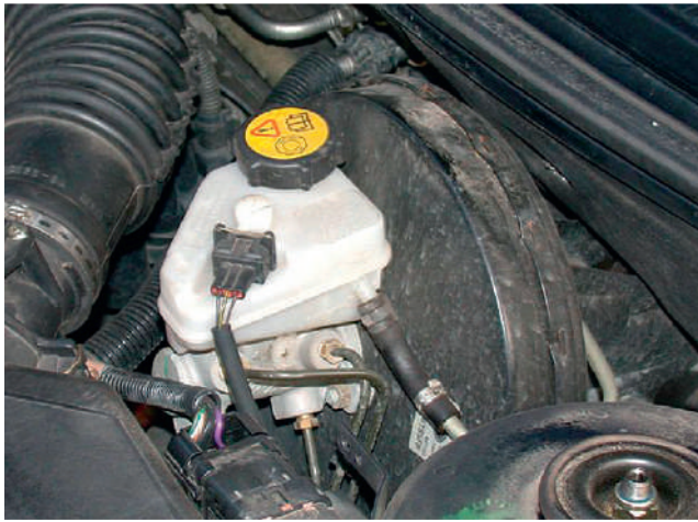
Figure 4.101 Master cylinder and fluid reservoir fitted on to the servo
